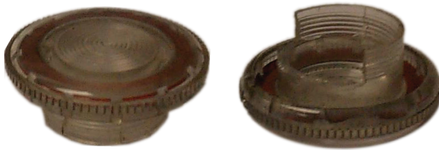
Damaged plastic actuating buttons
