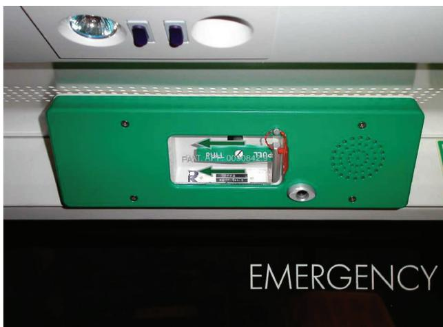
To prevent accidental operation, the 2 stage sliding cover is alarmed and, when opened initially to a stop, the alarm automatically activates.
